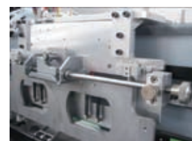
The carriage's height can be adjusted easily
