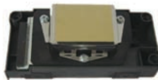
DX5 piezo printhead(24.5mm wide) with 8 lines of nozzles
